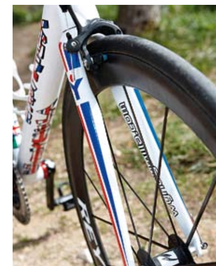
◀ The Dedacciai EDG fork is light, at a claimed 330g, and also very stiff for accurate handling
