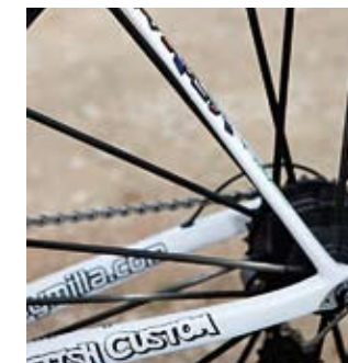
▼ Boxy chainstays and slim seatstays provide both power transfer and ride comfort
