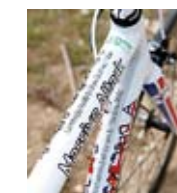
◀ The Dedacciai EDG fork is light, at a claimed 330g, and also very stiff for accurate handling
