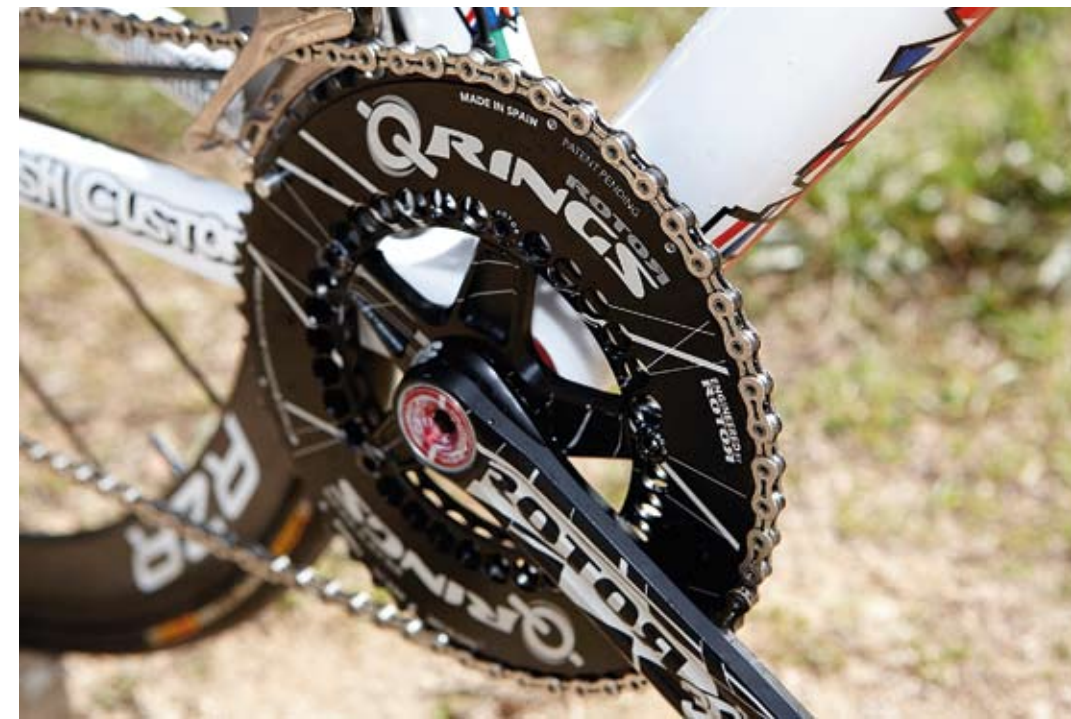
◀ Rotor's 3D+ cranks and aero, elliptical Q-rings are a stiff, power-enhancing combination
